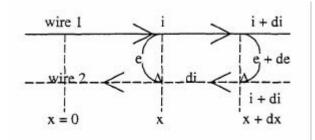
We use the simple relationships between voltage (e), current (I), capacitance per unit length (c) and inductance per unit length (L). The first equation relates the voltage change in the length dx to the current through it:
