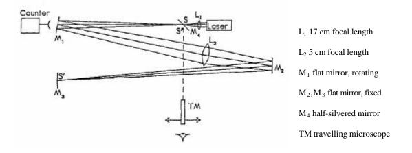
In an optimum arrangement the distance from the source (or object), S to the lens  $L_2$  is  $2f_2$ . An image S' is formed at M<sub>3</sub> and the image distance  $L_2$  to M<sub>3</sub> is then also  $2f_2$ . The distance from S to the rotating mirror M<sub>4</sub> should be approximately equal to  $f_2$  for best results.
