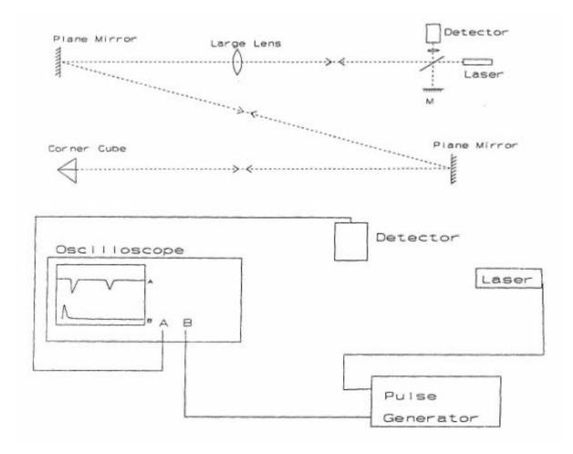
EXPERIMENT: Measure all relevant distances. Note that the retro-reflector may be placed in the beam anywhere beyond the large lens. You should do measurements for several different distances. Give some thought to where you position the cursor; some places may be better than others.
