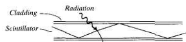
Figure 8.17 Cross section of a typical fiber scintillator. Some fraction of the emitted light is trapped by total internal reflection at the core-cladding interface.
