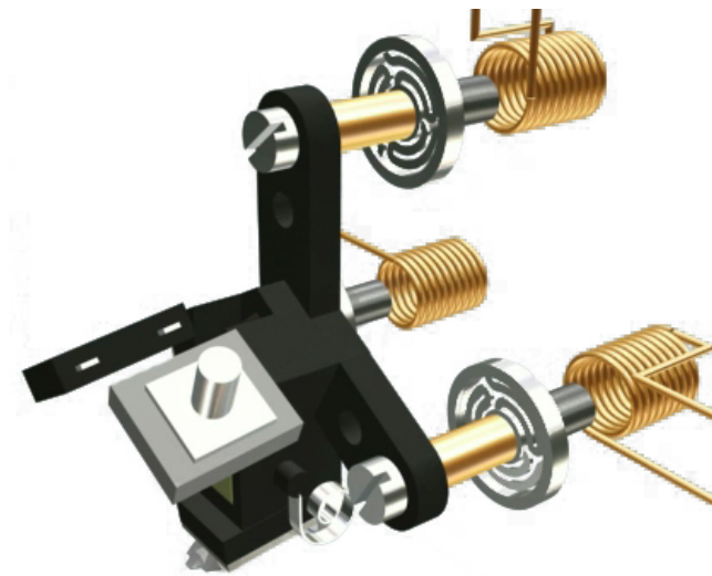
FIG. 2: A graphical representation of the tripod assembly part of the AFM, which holds the laser, the photodiode, the piezoelectric crystal, and the probe. Two of the circular springs can be seen with the 3 magnetic coils on each arm of the tripod, which are used to translate the probe assembly up, down, left, and right in fine detail using the feedback control loop.
