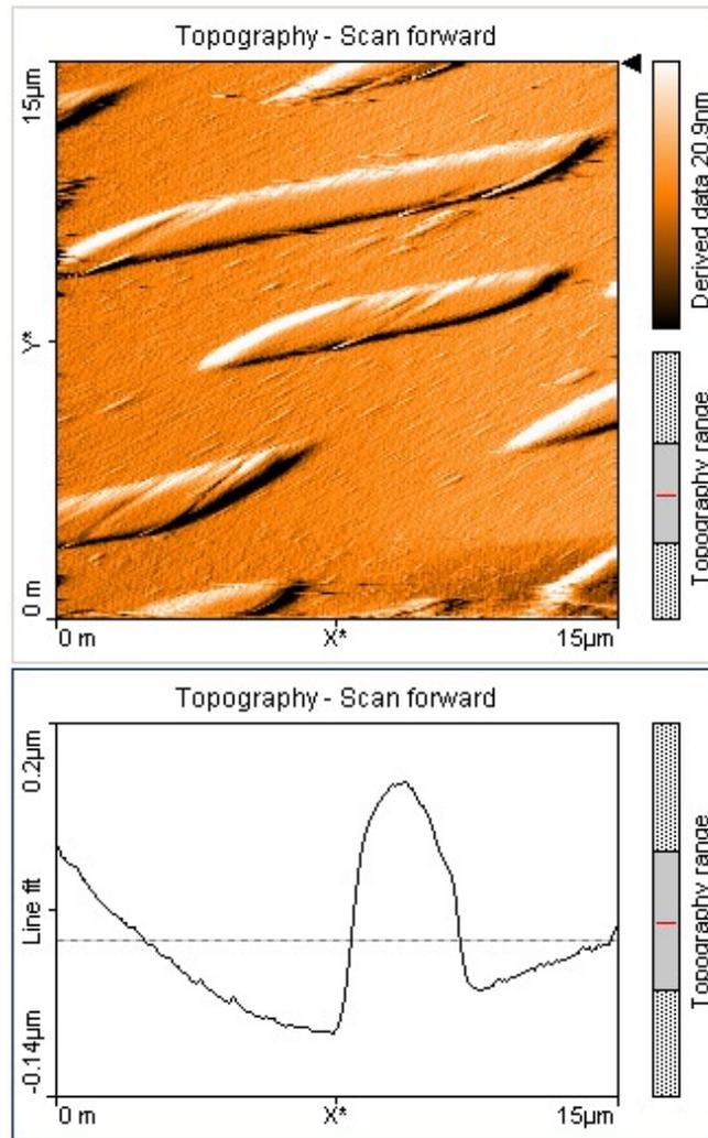
FIG. 4: Colour map and line graph showing the scan of a CD fragment
