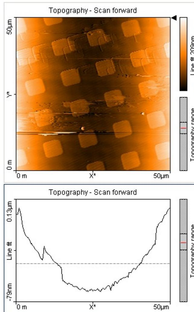
FIG. 1: Colour map and line graph representing  $10\mu$  AFM calibration grid
