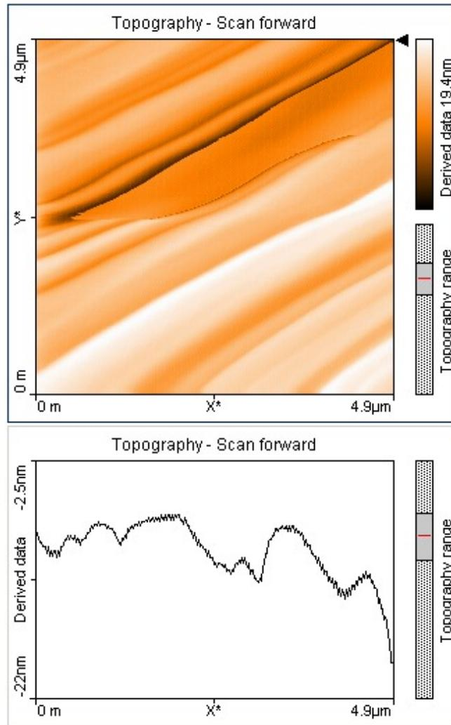
FIG. 6: Output for a small area of the gold plated diffraction grating
