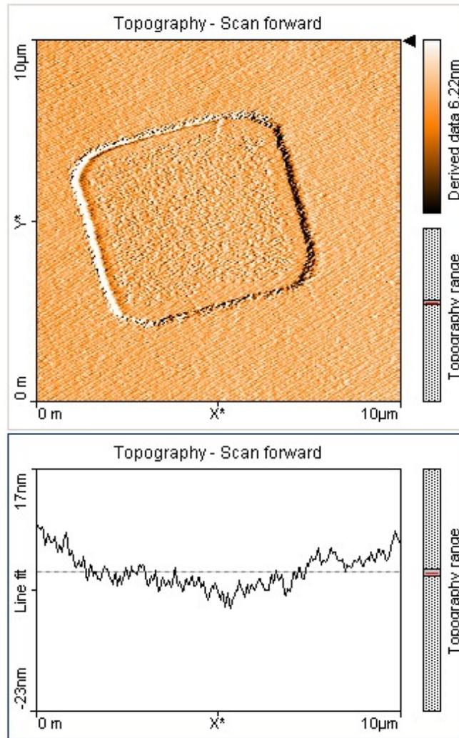
FIG. 3: Colour map and line graph showing a single square from the surface of the calibration grid
