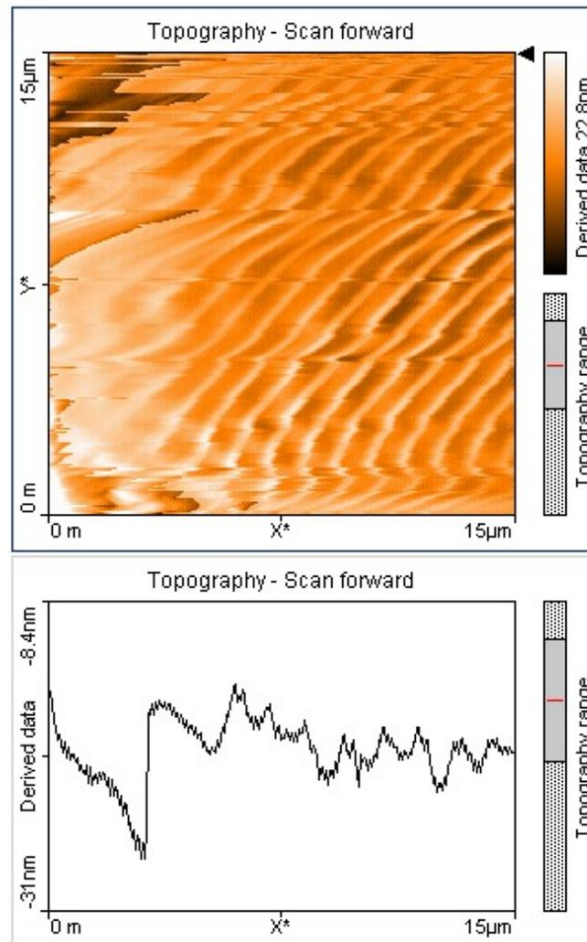
FIG. 5: Output from scan of gold plated diffraction grating.
